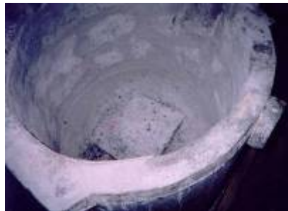
Ceramite® Tile Centered to Absorb Metal Impact
