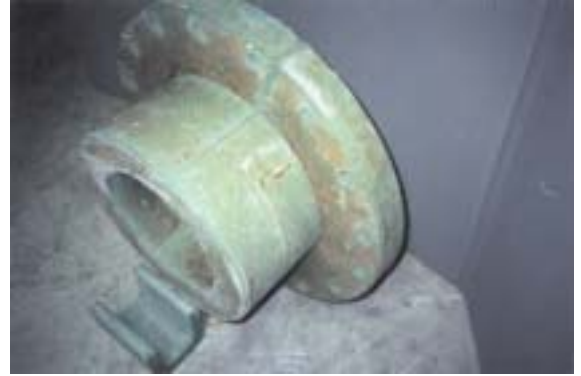
No.1 - HOLDING FURNACE OUTLET TIP ANODE FURNACE POURING TIP
