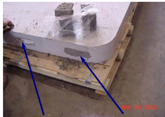
Rod Opening Packed With Ceramic Fibre to Offset Expansion
