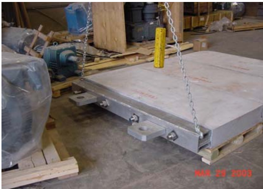
Lifting Assembly in Place
