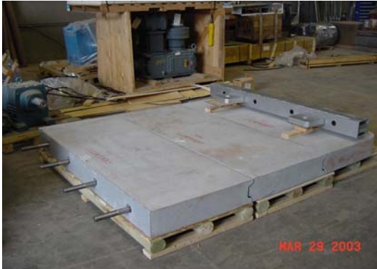
3 Piece Ceramite® Assembly With Stainless Attachment Rods
