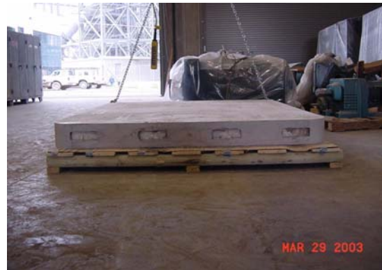
Opposite End of Lifting Assembly Opening for Stainless Rods & Supports
