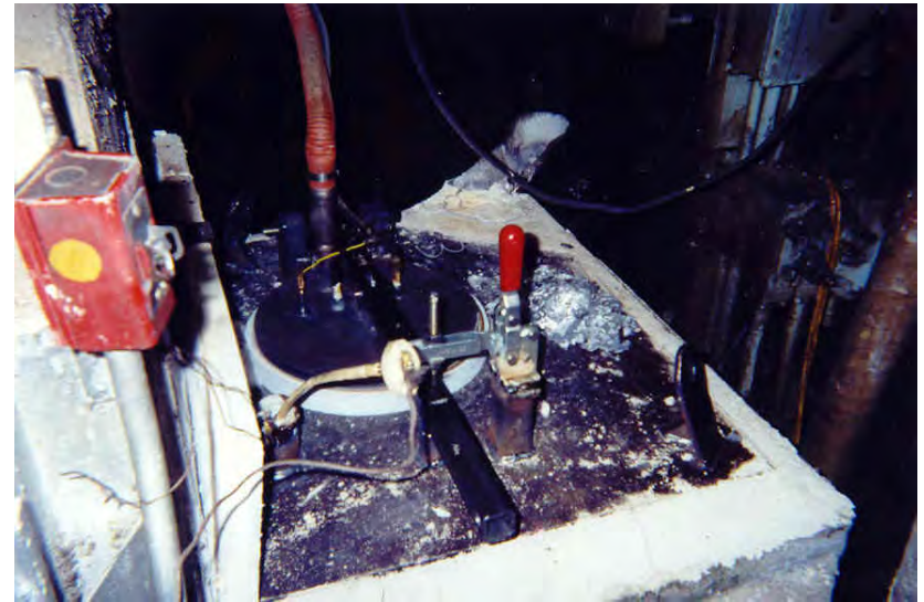
Ceramite® CSA Crucible in pump well position. Low pressure die cast operation.
