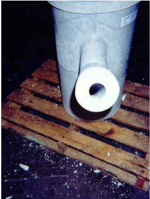
Discharge Snout of the Crucible This part replaced Vesuvius' Silicon Carbide.
